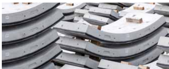
Curved HALFEN Cast-in channels in tunnel segments
